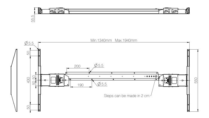
The Adjustable system includes a telescopic inner and outer rail where the base is welded on.
