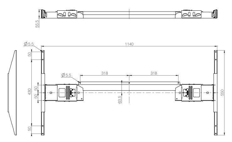
Compared to the Adjustable system the Fixed system only consists of one rail which is welded to the base in both ends.
