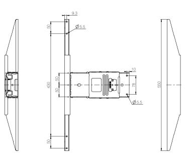
The Base system is without the inner and the outer rail. The system is preferred if the OEM want to weld his own rail on the Base, or if the desk design does not need a rail e.g. due to tabletop thickness. The Base system could also be used for a 3 leg desk.
