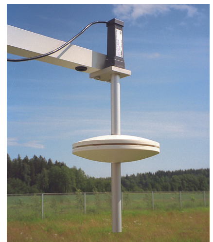
PTB210 paired with SPH10 static pressure head
