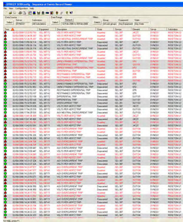
Figure 10 Combine SER Data From Multiple SEL-2440 DPAC devices for a System-Wide Log and Display
