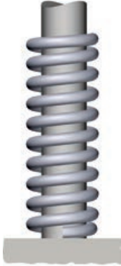
2. Not ground with internal location
