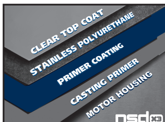
NSDX3 on Cast Iron
