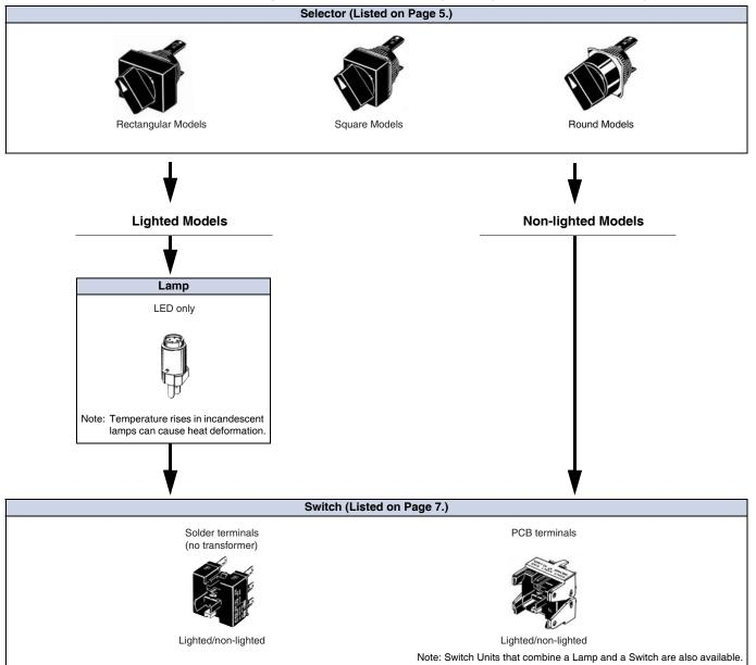
Ordering Individually ........ Selectors, Lamps, and Switches (Sockets) can be ordered separately. Combinations that are not available as sets can be created using individual Units. Also, store the parts as spares for maintenance and repairs. Selectors (Oil-resistant IP65 Models Only)
