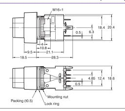
Rectangular A165W□-T Reduced-voltage lighting solder terminals (tab terminals #110)
